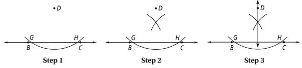
Construct a line perpendicular to line *n* and through point *X*. Sample answers shown.
